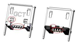
3. Change in shell & housing structure (Illustration below shows Shell stake 2.3mm version):
