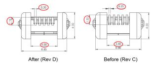
2. Change in shell & housing structure (Illustration below shows Shell stake 2.3mm version):
